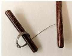
**Needle Tool** - designed to cut clay into strips, cut designs or texture in clay and create holes. The needle tool has a long sharp needle set in a heavier handle.
