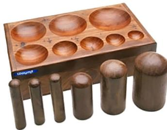
**Dapping block** - used to create a depression in flat metal. The block can be wood or metal and has concave depressions in it. A hammer or a die are used to force the metal down into the depression.
