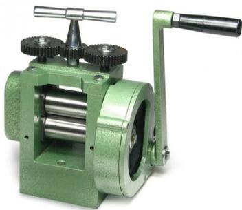
**Roller mill** - used to flatten and thin metal or to add texture to metal by rolling metal and fabric, leaves or other thin objects through the steel rollers
